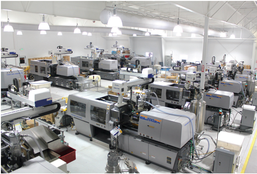
Prism sticks to all-electric machines, which avoids oil contamination and improves process control. A study showed the machines to be sensitive enough to run without cavity-pressure sensors.
